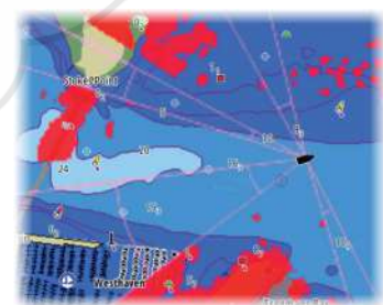
Radar Overlay on a Chart
