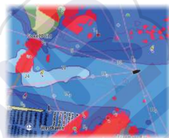
Radar overlay on a chart
